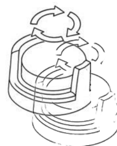
Lift the emergency stop
